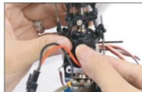
18. 将前后升降伺服器拉杆连上 Link up all the push-rods on the front & rear servoes.
