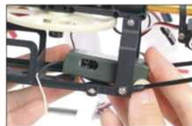
6. 将接收机放进机身并用双面贴粘好 Put the receiver into the body and stickup with double paste.
