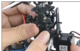
17. 将左右伺服器拉杆连上 Link up all the push-rods on the left right servoes.
