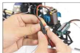
12. 将马达和调速器连接 Connect the motor with ESC.
