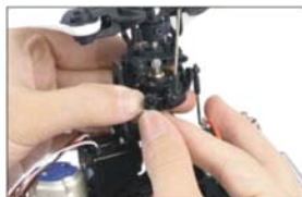
19. 将螺距伺服器拉杆连上 Link up the push-rods on the pitch servo.
