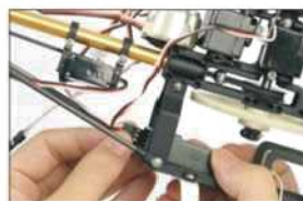
11. 将前后升降伺服器连接在第一通道 Connect the front & rear ELE servo with CH2
