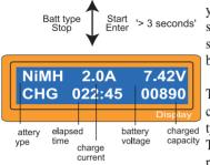
impedance and small capacity can lead to the higher charge current by the processor at automatic charge mode. But in 'Man' mode, it will charge the battery with the charge current you set at the display. Each mode can be switched by pressing INC or DEC button simultaneously when the current field is blinking.
