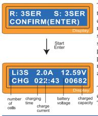
This shows the number of cells you set up and the processor detects. 'R:' shows the number of cells found by the charger and 'S:' is the number of cells selected by you at the previous screen. If both numbers are identical you can start charging by press Start/Enter button. If not press Batt Type/Stop button to go back to previous screen. Then carefully check the number of cells of the battery pack to charge again.
