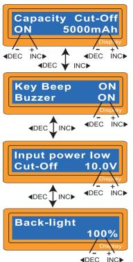
This program sets the maximum charge capacity that will be supplied to the battery during charge. If the delta-pack voltage is not detected nor the safety timer expired by any reason, this feature will automatically stop the process at the selected capacity value.
