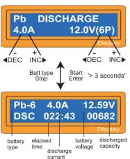
Set discharge current on the left and final voltage on the right. The discharge current ranges from 0.1 to 5.0A.
