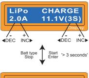
The left side of the first line shows the type of battery you select at the users setting. The value on the left side of second line sets a charge current and the value on the right side of second line sets the voltage of the battery pack.
