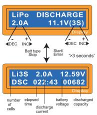
The value of discharge current on the left side of screen may not exceed 1C for a maximum safety and the final voltage on the right should not be under the voltage level that is recommended by the battery manufacturer to avoid deep discharging. To start to discharge, press Start/ Enter key for more than 3 seconds.
