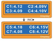
Using the individual connection cable to the battery, you can check the individual voltage of each cell in the battery pack. When connect the cable to the port on the right side of the charger the program shows them for maximum 8 cells in sequence. To utilise this feature, the battery pack must have output connector that linked to each cells.
