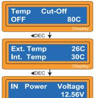
The internal temperature of the charger and the temperature of battery being charged.
