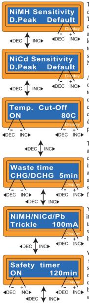
This shows the trigger voltage for automatic charge termination of NiMH and NiCd battery. The effective value ranges from 5 to 20mV per cell .If the trigger voltage is set higher, there is a danger of overcharging the battery; if it is set lower, there is a possibility of premature termination. Please refer the technical specification of the battery.(NiCd default:12mV NiMH default:7mV)
