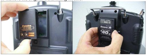
2.Put the Corona 2.4 Ghz transmitting module into the module port and screw on the transmitting ant
