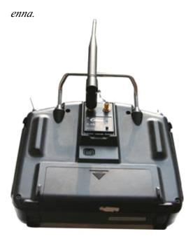
3. Turn the transmitter power on and check the RF power indicators on the module operate, and also on the radio.
